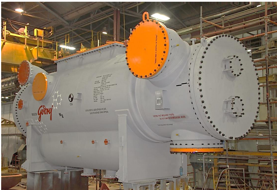
Steam Surface Condenser
